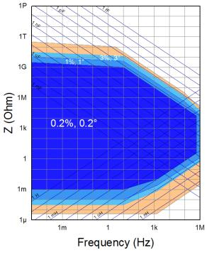
External high power boosters extend accuracy to 1  $\mu\Omega$  3T connections > 1k $\Omega$  , 4T otherwise •
