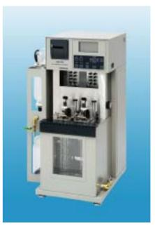
Model **AKV-202** has been designed for automatic determination of **KINEMATIC VISCOSITY**. Once a specimen is set the series of processes including timing, cleaning/drying of viscometer tube, and reporting are fully automated. AKV-202 is an economical bench-top system, which saves not only the technician's time but also valuable laboratory floor space and budget.
