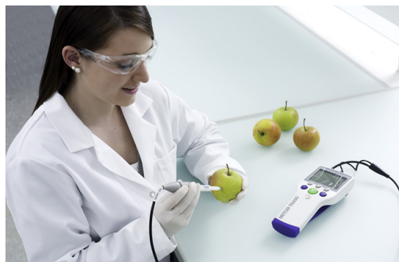
figure 2: use of a portable pH meter with puncture electrode to check pH value of apples
