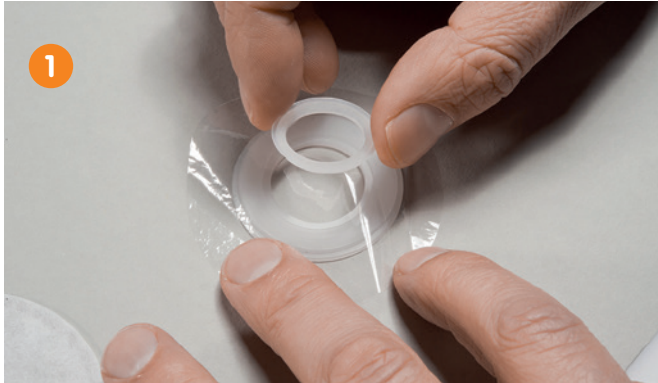
1 Prepare small-mass holder for small amounts of sample.
