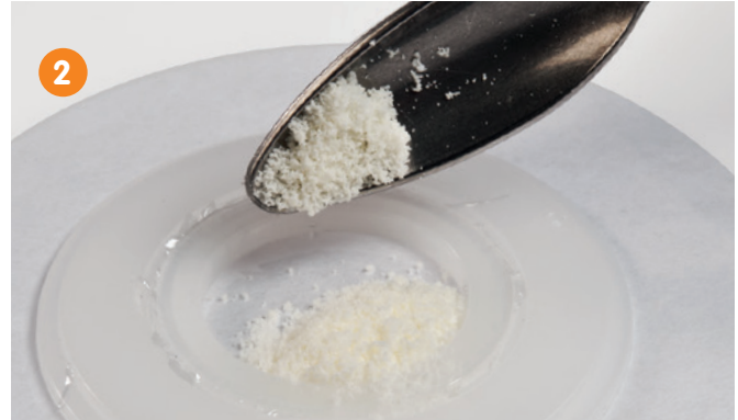
2 Fill small-mass holder with typically 100 – 200 mg sample.
