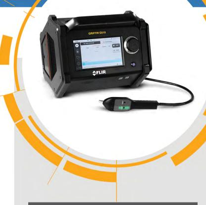
THE GRIFFIN G510 GAS CHROMATOGRAPH MASS SPECTROMETER (GC/MS) IS A VERSATILE, PERSON PORTABLE CHEMICAL IDENTIFIER. IT COMPLEMENTS PRESUMPTIVE TECHNIQUES USED DURING EMERGENCY MISSIONS, BY ENABLING RESPONDERS TO ANALYZE ALL PHASES OF MATTER (LIQUID, SOLID, VAPOR) AND BY PERFORMING RAPID FIELD-CONFIRMATION OF CHEMICAL HAZARDS.
