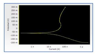
PARSTAT4000A Tafel plot experiment in K0047 Corrosion Cell as described in ASTM
