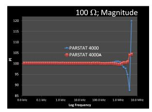
PARSTAT 4000A Magnitude impedance plot on a 100  $\Omega$  resistor using standard cable.
