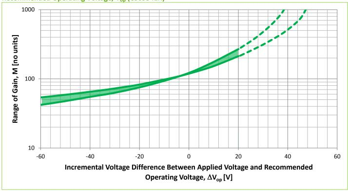
Figure 12 – Variation of Gain as a function of Difference between Actual Applied Operating Voltage and Recommended Operating Voltage,  $V_{op}$  (C30955EH)
