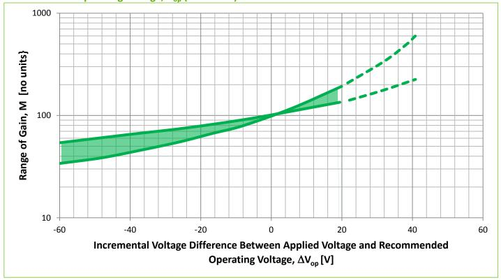
Figure 13 – Variation of Gain as a function of Difference between Actual Applied Operating Voltage and Recommended Operating Voltage, V<sub>op</sub> (C30956EH)
