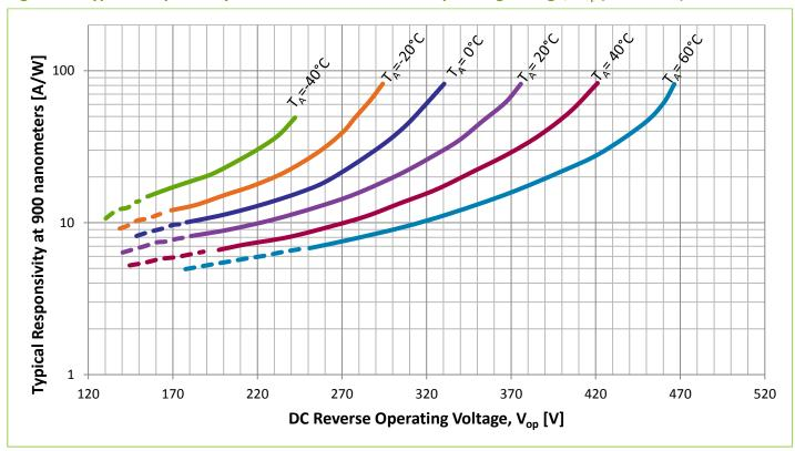
Figure 4 – Typical Responsivity at 900 nm as a function of Operating Voltage, V<sub>op</sub> (C30956EH)
