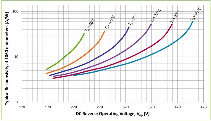
Figure 7 – Typical Responsivity at 1060 nm as a function of Operating Voltage, V<sub>op</sub> (C309556EH)
