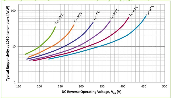
Figure 6 – Typical Responsivity at 1060 nm as a function of Operating Voltage, V<sub>op</sub> (C30955EH)
