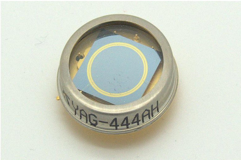
The YAG series high-performance Si PIN photodiodes are well-suited for applications using 1064 nm (YAG) lasers.
