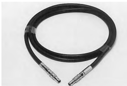
LL174 Signal Cables RG-174 50- \Omega Cable with two LEMO male plugs. LL174-0 0.1-m length LL174-1 0.25-m length LL174-2 0.5-m length LL174-3 1-m length LL174-4 2-m length
