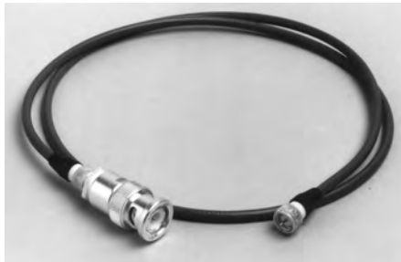
C-19-2 Microdot 100-Ω Miniature Cable with one BNC male plug and one microdot male plug; 0.61-m (2-ft) length.
