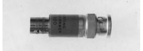
IT100 Inverting Transformer A compact pulse-inverting transformer for use in a 50- \Omega system; has low distortion; good linearity, freedom from overload effects, 0.8-ns rise time capability, and 7% tilt in 100 ns.
