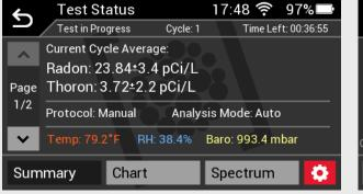
Alpha spectrometry measurements are used to determine radon and thoron concentrations:
