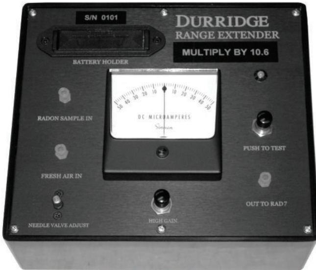
Figure 21: The DURRIDGE Range Extender reduces the radon concentration delivered to the RAD7 by a factor of 10. The RAD7 pump can cycle on and off without affecting the reduction factor.
