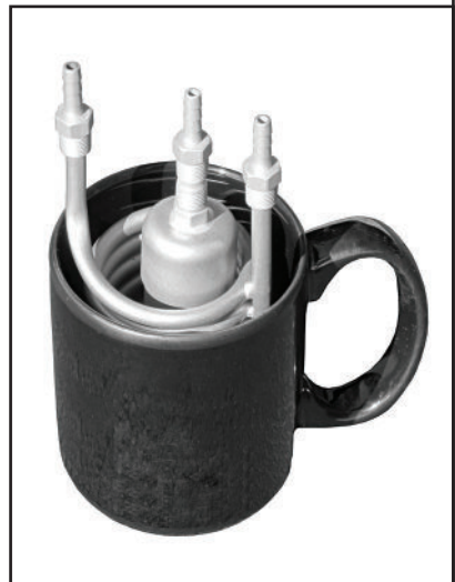
Figure 25 (Below): The Cool Trap is placed in a vessel containing icy water.
